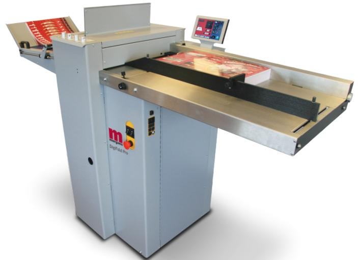
The maximum sheet size is 700mm x 385mm (900mm x 385mm with optional extension table) allowing a wider range of jobs to be tackled. Perforation is also standard on the DigiFold Pro with up to 5 perforation wheels being used across the sheet.
