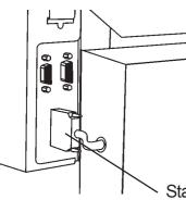
The SquareFold is equipped with a stacker full sensor. In mode 1 and 2, stacker full signal appears 30 booklets after the stacker full sensor has been blocked. In mode 3 and Bypass, stacker full signal appears 20 booklets after the stacker full sensor has been blocked. Whenever the books are removed the count starts from zero again. If the stacker full function is not desired, disconnect the stacker full plug from its receptacle.
