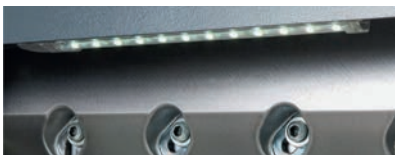
LED cutting line indicator ensure optimum illumination, even when lighting is poor.
