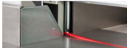
A cutting stick ejector eases and abbreviates the knife change.
