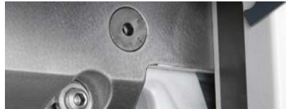
Knife depth can be conveniently adjusted from the front.
