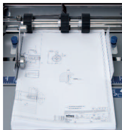
Movable feeding roller (left) for an optimal feeding for cross fold
