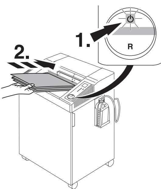
Is the rocker switch (1.) pressed? The green light rocker switch is ON? (1.).
