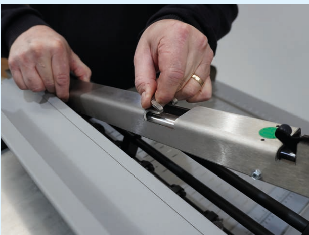
Images above, showing the removal of the 'EasyBlade' safety cover.
