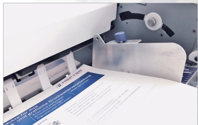
500 sheet feeding tray with the ability to count and pause job.
