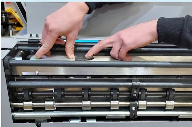
*EasyBlade quick release mechanism.*
