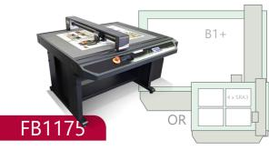
**Premium Arch B1+ or 4 x SRA3 creasing and cutting system** The FB1175 is the largest cutting table in the range, handling media up to B1+  $(800 \times 1100 \text{mm})$ , with a maximum effective cutting area of up to 750 x 1095 mm.
