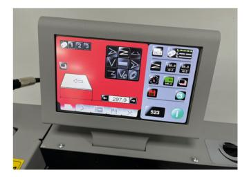
A user friendly SmartScreen panel enables adjustments to 0.1mm on the fly if the fold plates or delivery roller needs to be moved. Within this SmartScreen panel are a counter and batching facility which are standard features. A further feature of the sophisticated SmartScreen is the ability to memorise and store repeated jobs in the alpha numeric memory which can then be retrieved within seconds.
