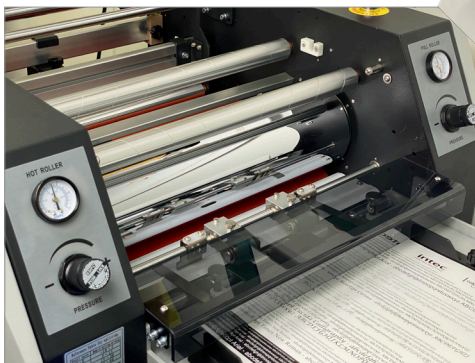
Premium oil heated, high gloss chromium roller, for mirror finish results
