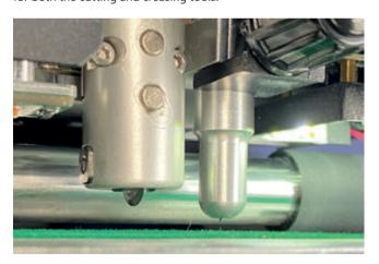
This combination of tools provides a much wider media handling capability and more defined, smoother crease for thick card up to 450 micron. The individual tool actions are controlled via the included ColorCut Pro 5 Production Studio software.
