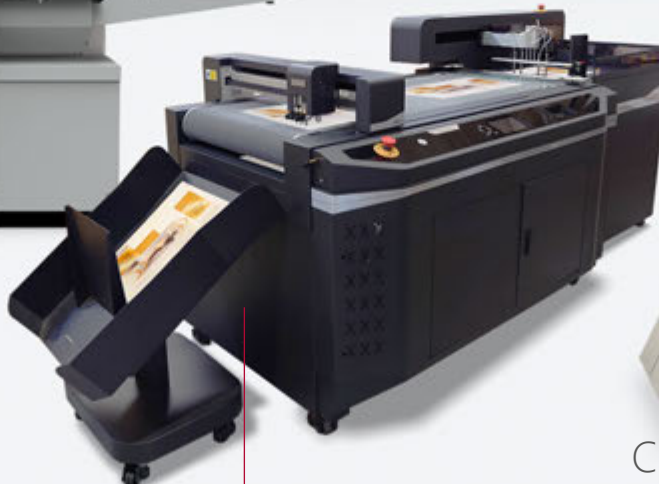
FB9550 Automated digital die cutter
