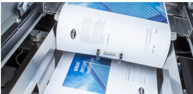
Collating station with the tumbler mechanism prepares the book for stapling and folding
