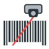
The system supports DataMatrix and PDF417 codes (up to 24 characters each), with a minimum barcode feature size of 0.3 mm for dependable, high-resolution reading.
